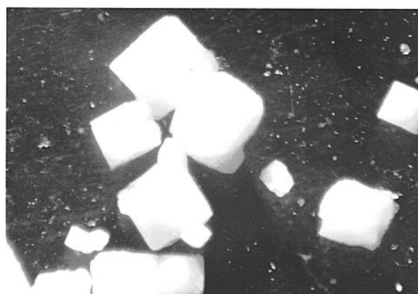
Fig. 3 Optical micrographs of crystals of SSCPD before and after rehydration using a 0.85 \text{ g cm}^{-3} \text{H}_2\text{O}_2 solution for 4 days
